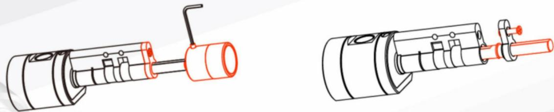
1. According to the above figure, use Allen Wrench to remove **Knob**① by loosening the screw on **Knob**①. And use a screwdriver to loosen Short Screw M4⑦ on Short **Cover**④, and then remove **Short Cover**④ and **Spindle**②.
